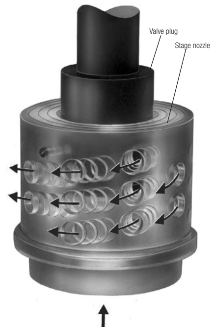
Flow through ZK 29 radial stage nozzle
